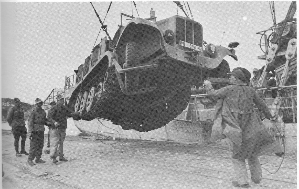
Used in substantial numbers for towing medium and heavy artillery, German half-track tractors are being taken off boats. Vehicle shown is a 5-ton medium artillery tractor.
