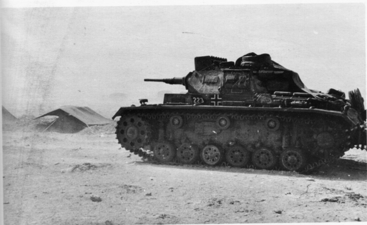
An Ausfuehrung F of the Panzer III, recognizable by its final drive and idler wheels. Jerry cans stored on the turret roof contain water.
