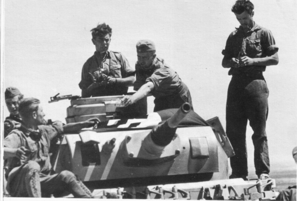
The tank which did most of the fighting on the German side during the initial phases of the campaign was the Panzer III. Initially equipped with a 37 mm gun, vehicles used in Africa generally had the 50 mm KwK L/42. Later German tanks had a five-man crew.
