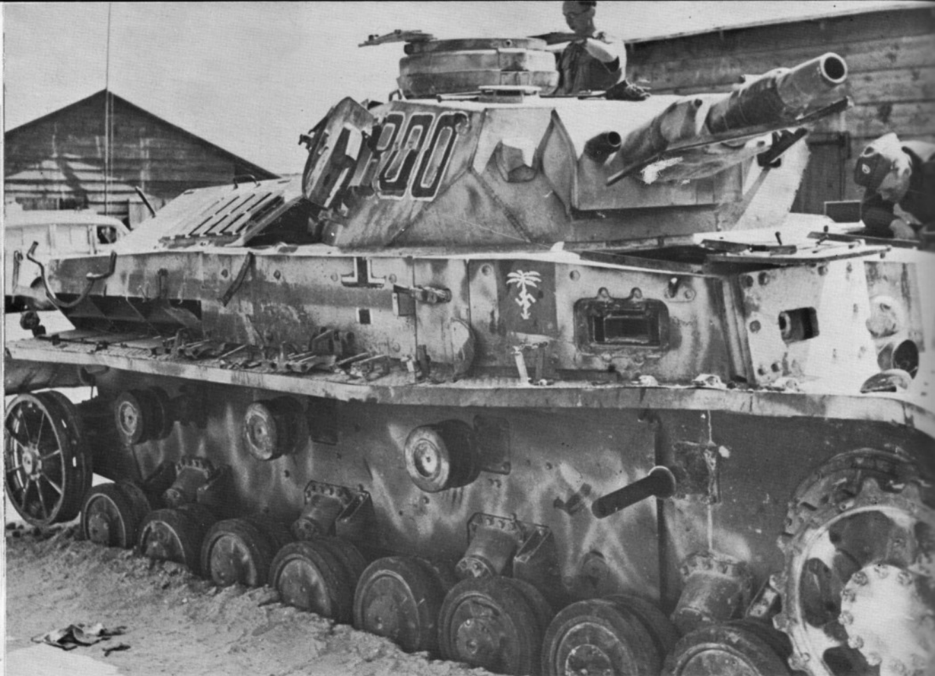
This is an E version of the Panzer IV, with the distinctive step-like frontal plate, protected subsequently by additional armor.
