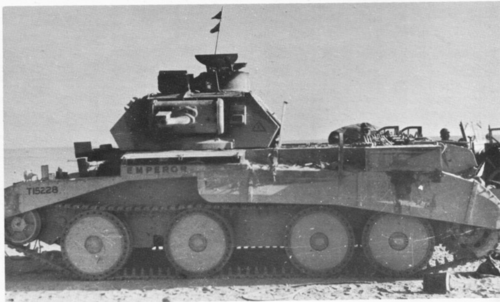
The long series of "Cruiser" tanks encountered in Africa led by this Mark IV A, a vehicle equipped with a 40 mm gun. They were fast but technically not too reliable.
