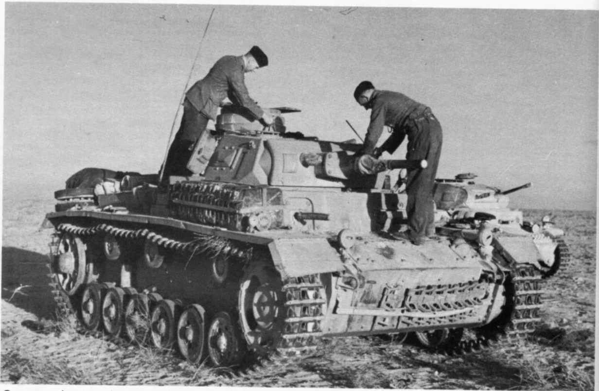
Crew members readying a Panzer III for further action. The abrasive impact of the desert sand necessitated tight closing of all openings. Spare track links were carried on the front plate to afford additional protection.
