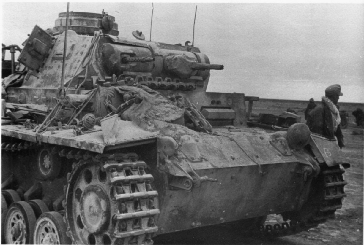
The command version of the Panzer III carried a dummy main armament and had one MG 34 installed in the mantlet of its fixed turret. This vehicle had obviously received a hit which did not penetrate.
