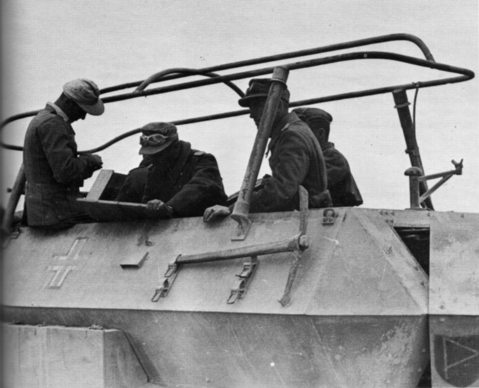
Armored half-tracks also served as vital communication centers to guide armored forces widely scattered throughout the desert. Note the typical frame antenna used on most armored radio vehicles of this period.
