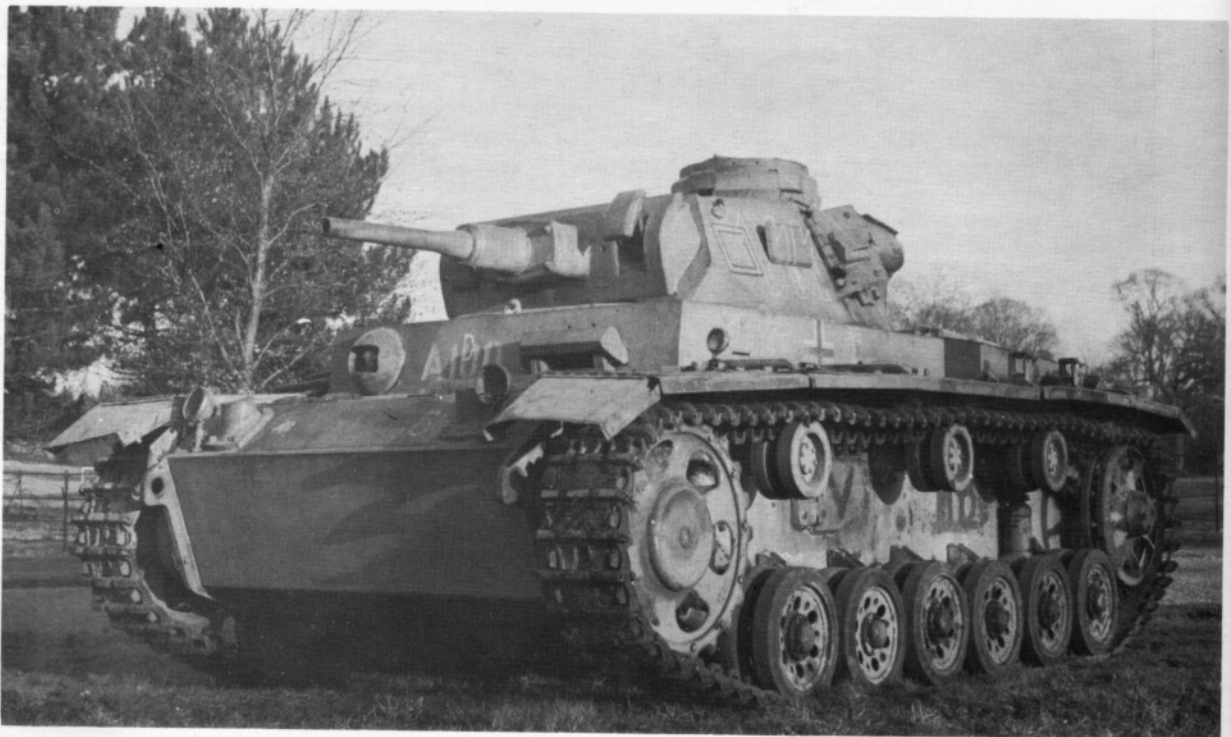
This is the Ausf. H of the same vehicle. Note the difference in final drive and idler wheels and also the different spacing of the return rollers. 400 mm tracks were used for the first time.
