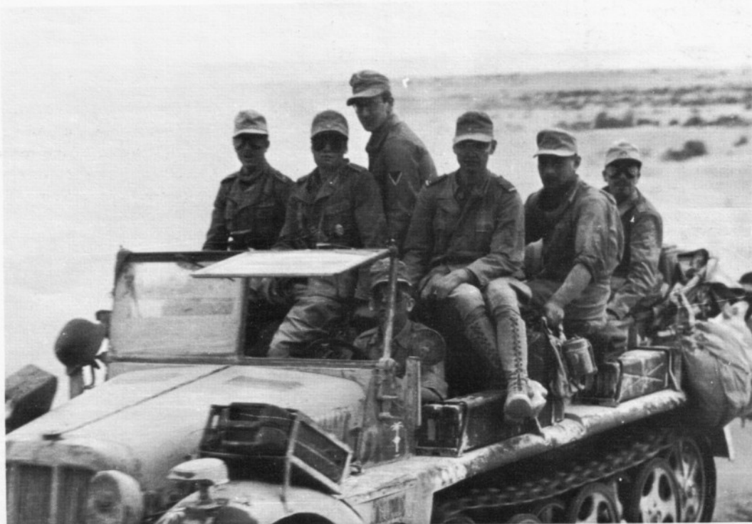
The smallest of the German half-track tractors used in Africa was the 1-ton Zgkw. It was the main prime mover for anti-tank guns and also served as a troop carrier.
