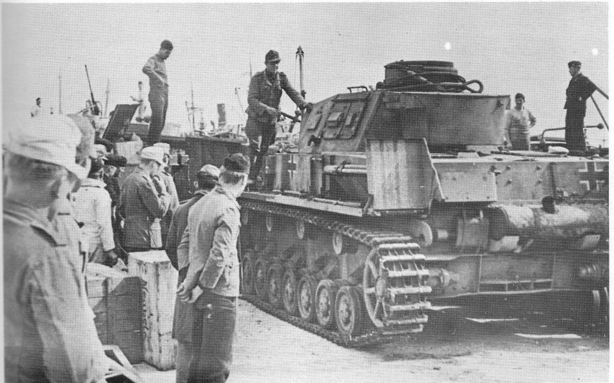
A Panzer IV has just been put on a pier in North Africa. This is an F version of one of the most versatile fighting vehicles of the German armored force.
