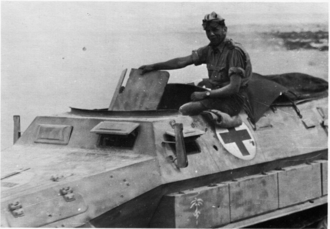
Armored ambulances served friend and foe alike. Note the absence of any armament on these vehicles. Basic vehicle was the standard 3-ton armored personnel carrier, a half-track vehicle.
