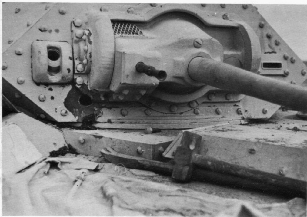
The impact of German tank and anti-tank weapons is clearly demonstrated by this penetration of a 50 mm shell right below the gun mantlet.
