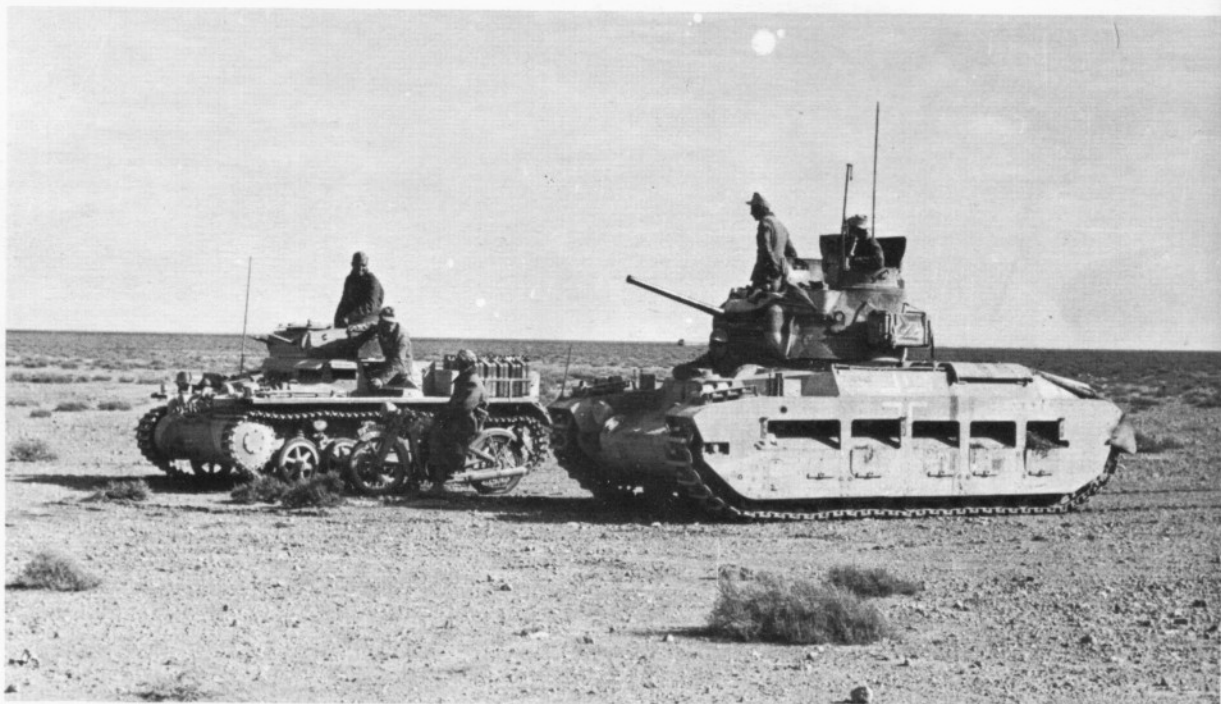
During their first encounters, a number of British fighting vehicles fell into German hands. Picture shows a captured British "Matilda" Infantry tank, accompanying a German Panzer I, a light vehicle never intended to be used as a fighting vehicle.
