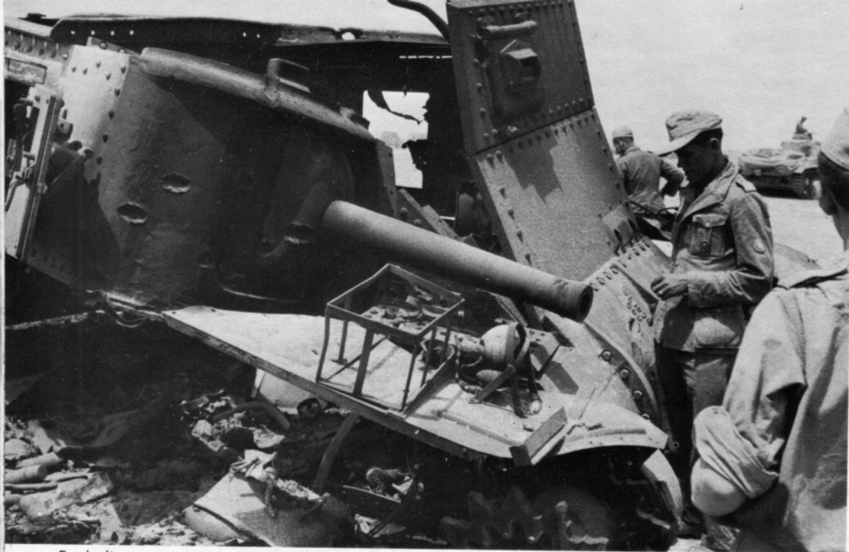
Exploding ammunition left nothing but a pile of junk iron of this M 3 tank. Note the limited traverse provided for the 75 mm gun. Its heavy armor protected it against smaller German weapons.
