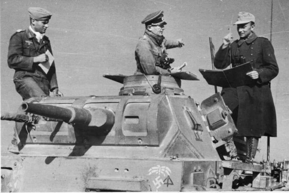
Some of the early 37 mm vehicles of the Panzer III series, the Ausf. E, carried two machine guns in the gun mantlet. They were used exclusively by staff officers and for observation purposes. Note the insignia of the Afrika-Korps painted beside the driver vision slot. The vehicle belonged to the 15th Panzer Division.
